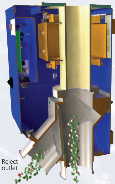
Cross section of E-Z Tec 9100 showing principle of operation
